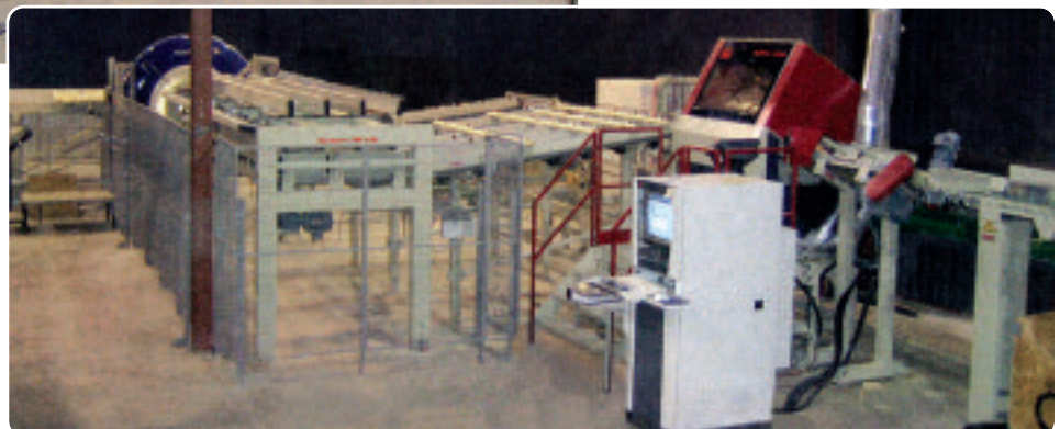
Rough mill line – automated infeed, material handling, optimizing, cross-cut saw and automated reject stations.
