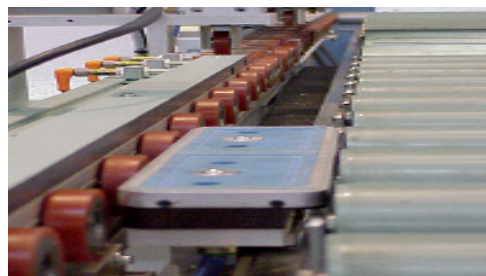
Suction cup clamping and moving system.
