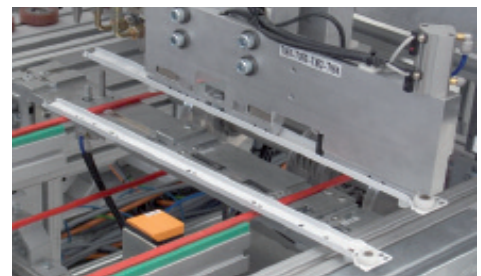
Drawer slide inserting station.
